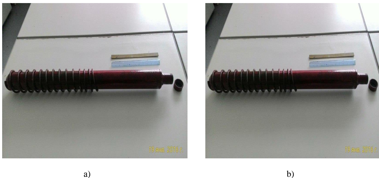
Figure 2. Ring energy divider in the manufacturing process (a); preparation for filling with coolant (b).
