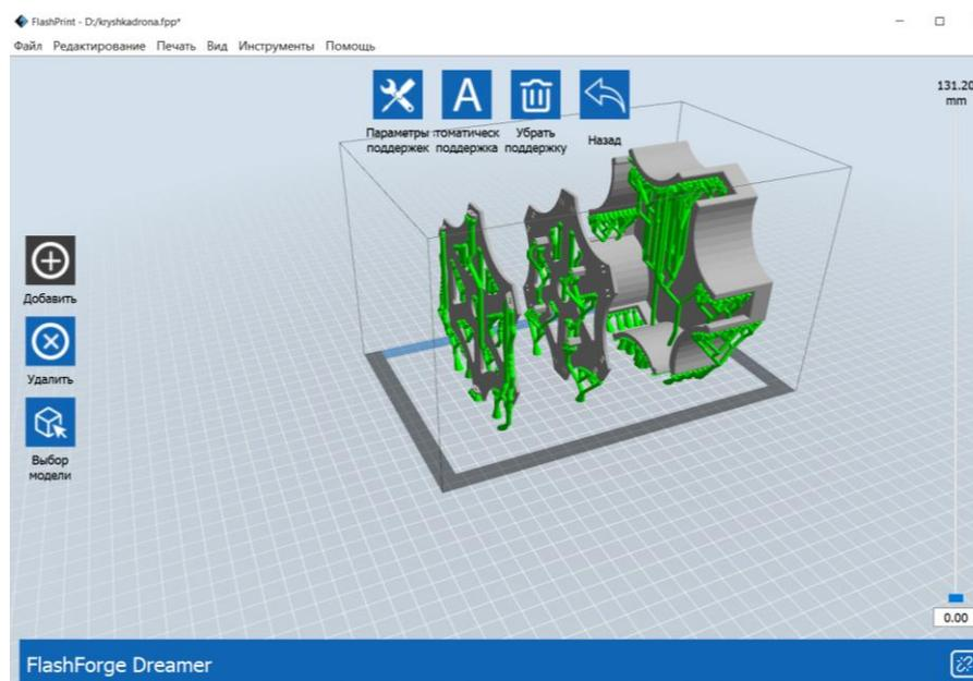
Figure 5. Support model for main parts of the corpus
