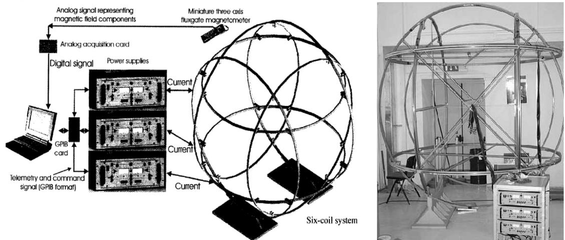
1.13 Fig. Geomagnetic field Simulator at the University of Federico II of Naples
