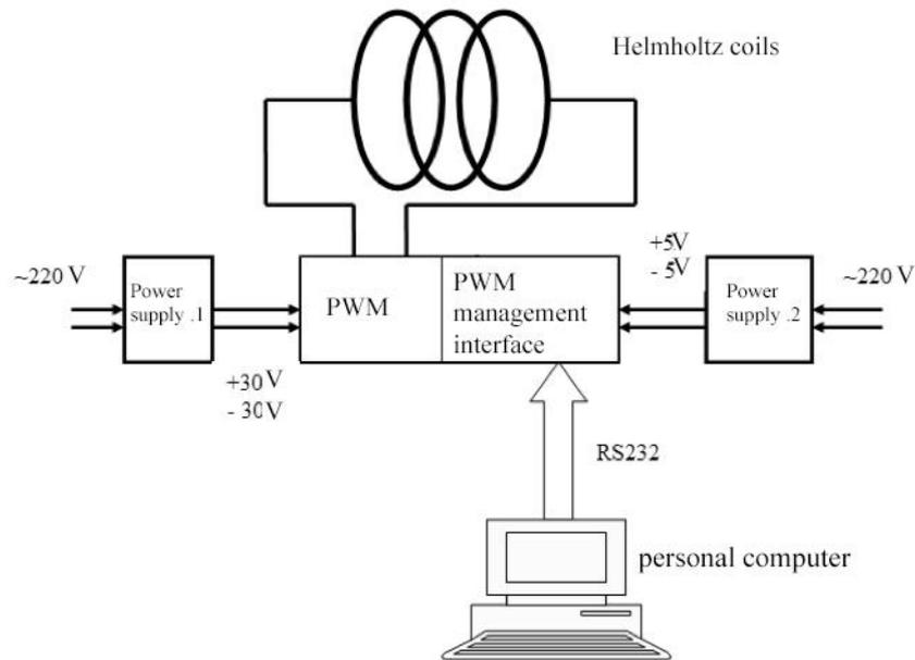
2.9 Fig. - The control circuit coils of the geomagnetic field simulator
