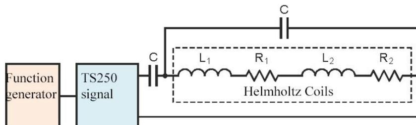
2.8 Fig. - formation of a high-frequency Helmholtz field using resonant current amplification to double the magnetic field.
