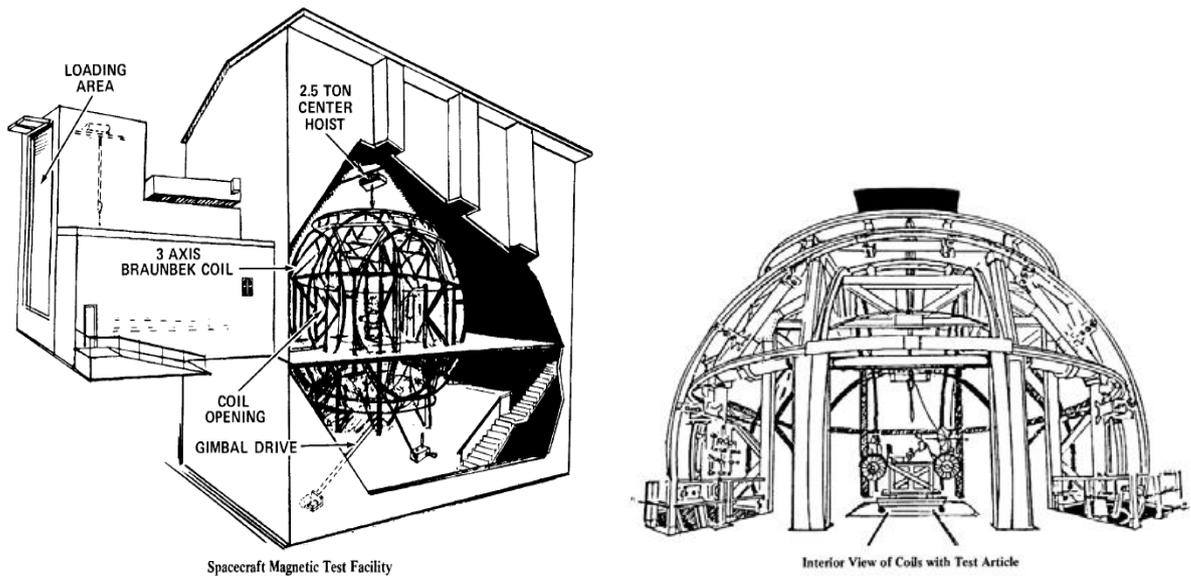
1.3 Fig. – General view of the geomagnetic field simulator in the Goddard Center, USA
