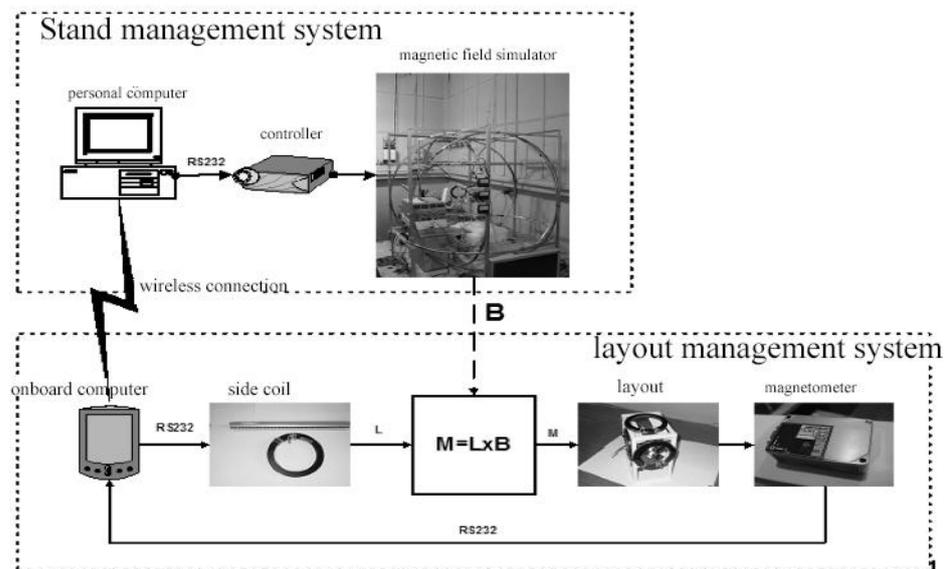
3.1 Fig.- scheme of functioning of the semi-natural modeling stand
