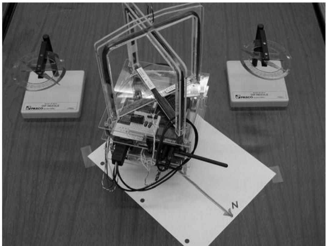
1.7 Fig. - Layout in USNA for testing the magnetic stabilization system
