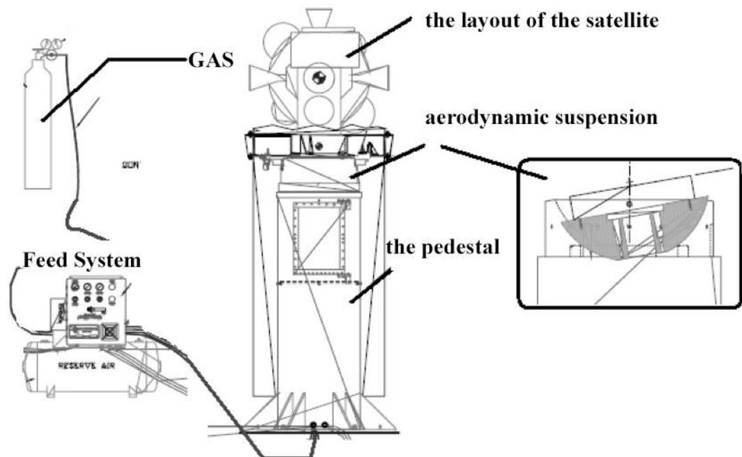
1.1 Fig.–The principle of operation of an aerodynamic suspension
