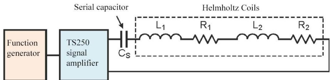
2.6 Fig. - at the resonance frequency, the generator signal amplifier gives a large current to the Helmholtz coils.
