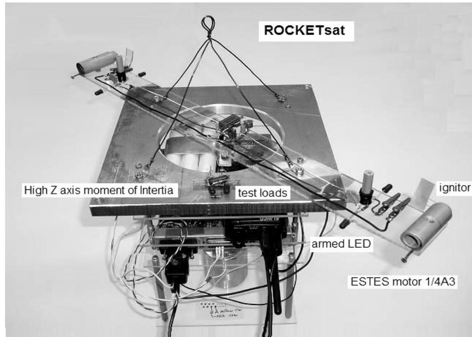
1.6 Fig.- Layout in USNA for testing micro-jet engines
