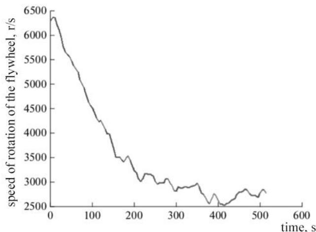
3.5 Fig. - evolution of the speed of rotation of the flywheels during the operation of the unloading algorithm
