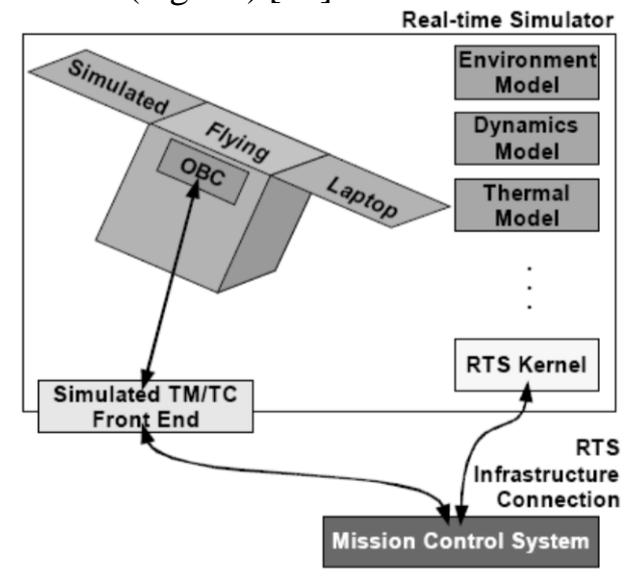
2.2 Fig. - The scheme of simulation of a control system of the Flying Laptop
