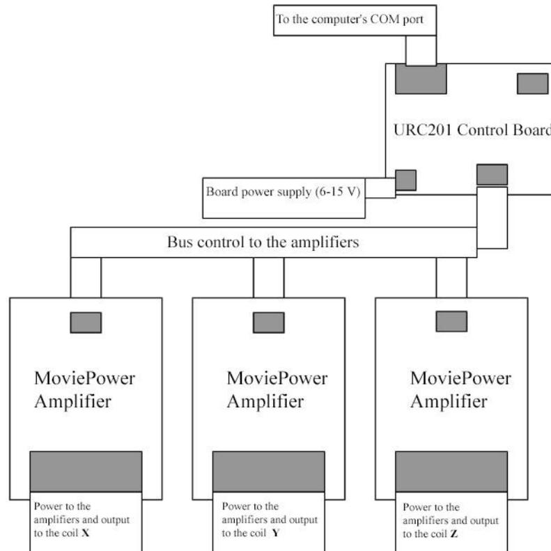
2.10 Fig. -the control Board (left) and connection diagram of PWM amplifiers and control Board URC201
