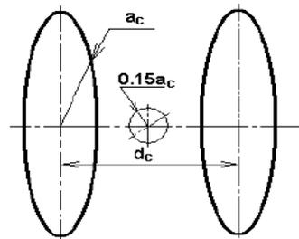
2.8 Fig. - determination of the homogeneity zone of the modeled field
