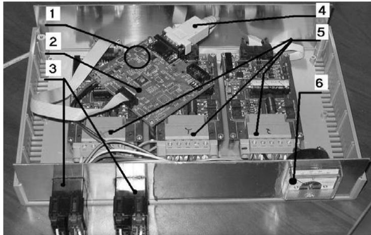
2.11 Fig.- the control unit of the coils of the stand. (1) - LED indicators of the control board; (2) - control board; (3) - power cable; (4) - PC control cable; (5) - power amplifiers; (6) voltage indicator.
