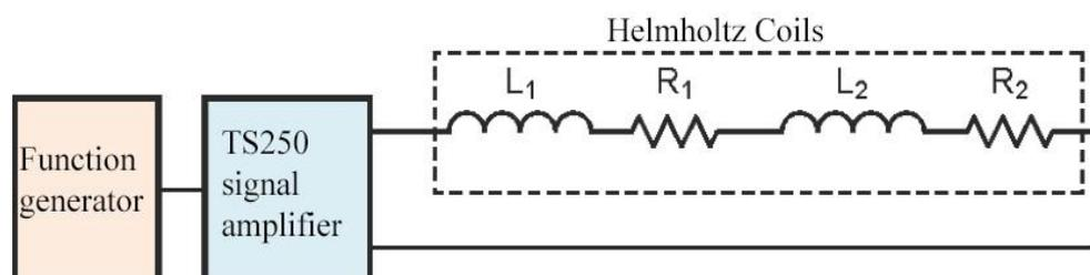
2.5 Fig. - representation of a circuit in which a generator signal amplifier directly controls a pair of series-connected Helmholtz coils.
