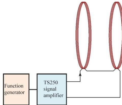
2.4 Figure – The TS250 generator signal amplifier controls a pair of Helmholtz coils.
