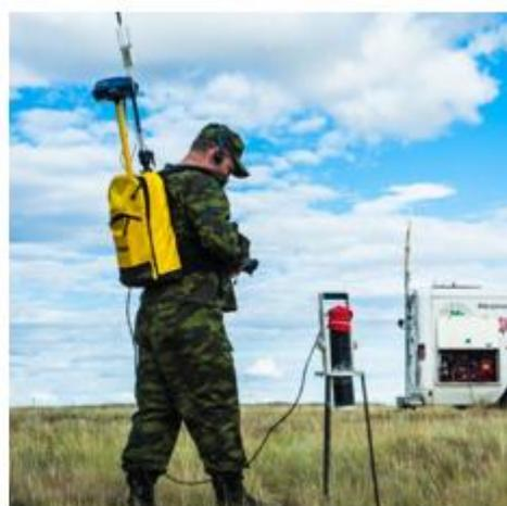
Figure 2 - Seismic survey (a) and coordinates determination of boreholes by GPS receivers (b)
