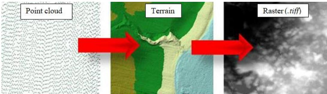
Figure 3 - The process of developing the ground surface model
