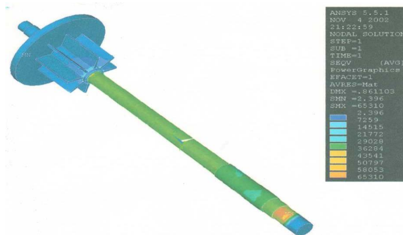
Figure 6 - Equivalent stress distribution
