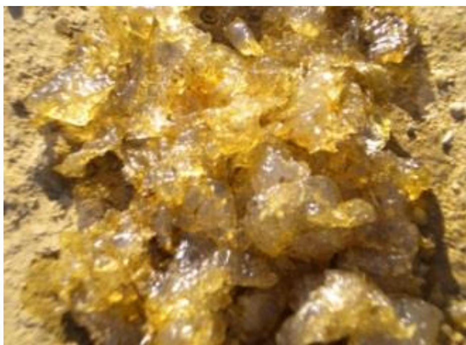
Figure 24 – Gellan solution after contacting with Kumkol ( 73 \text{ g}\cdot\text{L}^{-1} ) brine.
