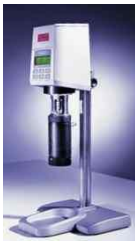
Figure 20 – Rheological viscometer Rheolab QC, Anton Paar (Austria).
