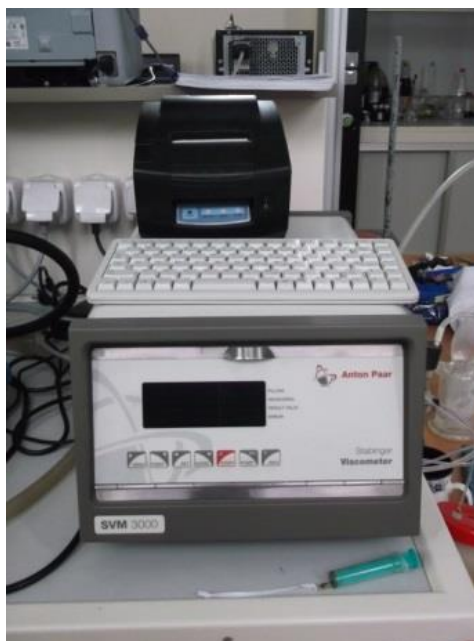
Figure 16 - Viscometer of Stabinger SVM 3000.
