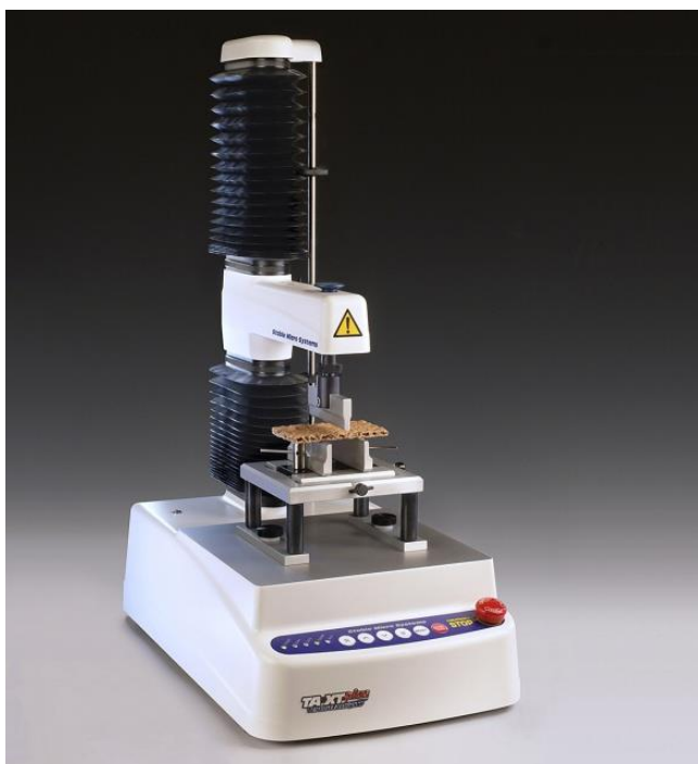
Figure 21 - Texture analyser TA.XT plus, Stable Micro Systems, (UK).
