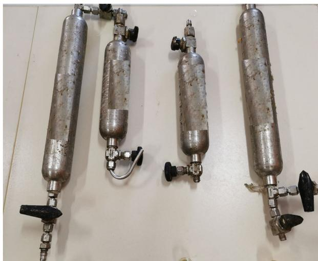
Figure 4.2 — Pressurized cylinders for a polymer solution sampling at the wellhead
