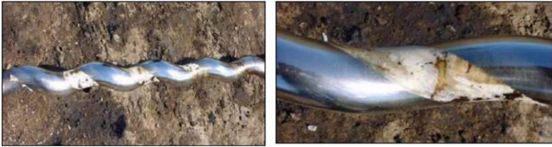
Figure 2.4 — Scaling PCP rotors in Daqing ASP flooding area [105]
